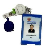
RFID card linked with BLE tag in white and the connected to hip thru Retractable Reel ID Card Holder .
